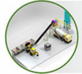
Concrete Batching & Mixing Plant
